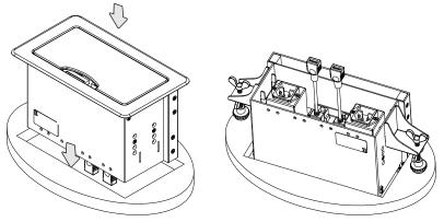
Figure 5: Inserting TBUS-6xl into the Prepared Opening
