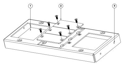
Figure 2: TBUS-6xl Inner Frame (P/N: 80-004499)
