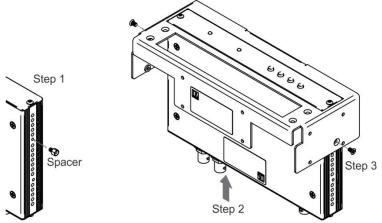
Figure 3: Installing the MegaTOOL
