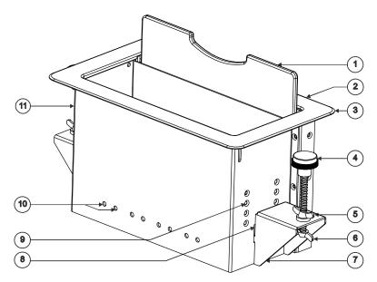
Figure 1: TBUS-6xl Enclosure Top View
